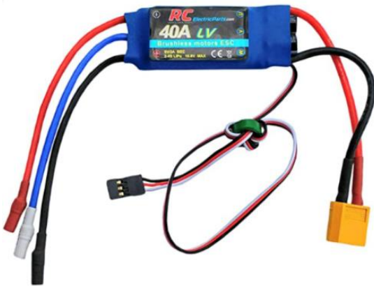
Figure 14: RC Motor Controller
